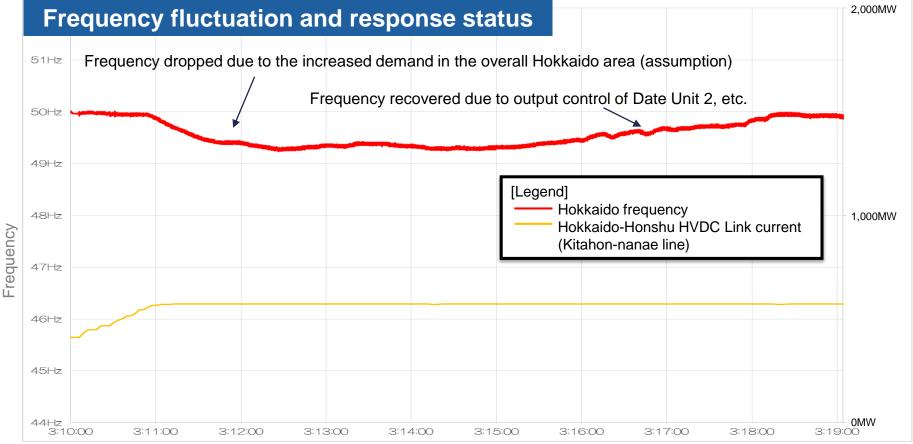
II. Sequence of Events from the Occurrence of the Earthquake to the Blackout 15 Immediately after the earthquake [2]-2 Overview (Tomato-atsuma Unit 1 output decrease – second load shedding)
