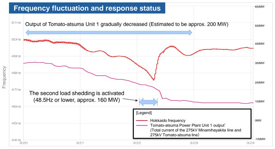
\* The transmission line current (Minamihayakita line + Tomato-atsuma line) value was almost twice as much as the generating-end output of Tomato 1G, starting around 3:08. Since it may have been caused by measurement abnormality of the generator, we used the transmission line current value.
