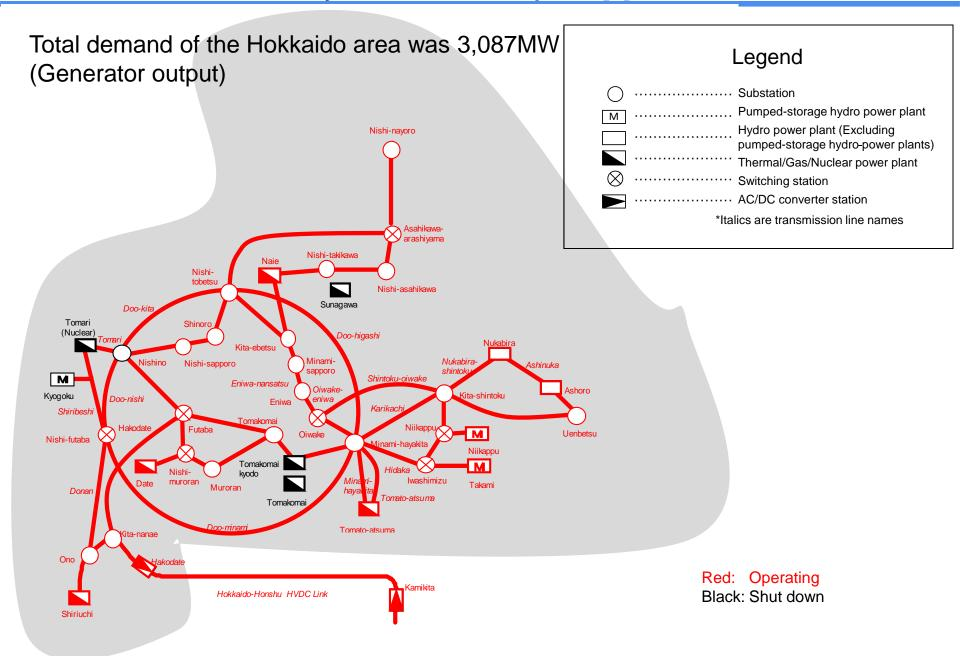
II. Sequence of Events from the Occurrence of the Earthquake to the Blackout Grid status immediately before the earthquake [0]
