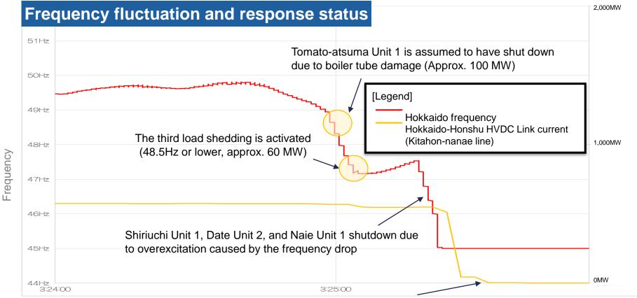
Hokkaido-Honshu HVDC Link disconnected (caused by frequency drop)
