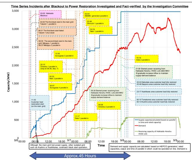
Black start operation was conducted as per the manual without obvious human errors. We have confirmed that there is a limit to the shortening of recovery time since generators could only gradually start beginning with small grids.
