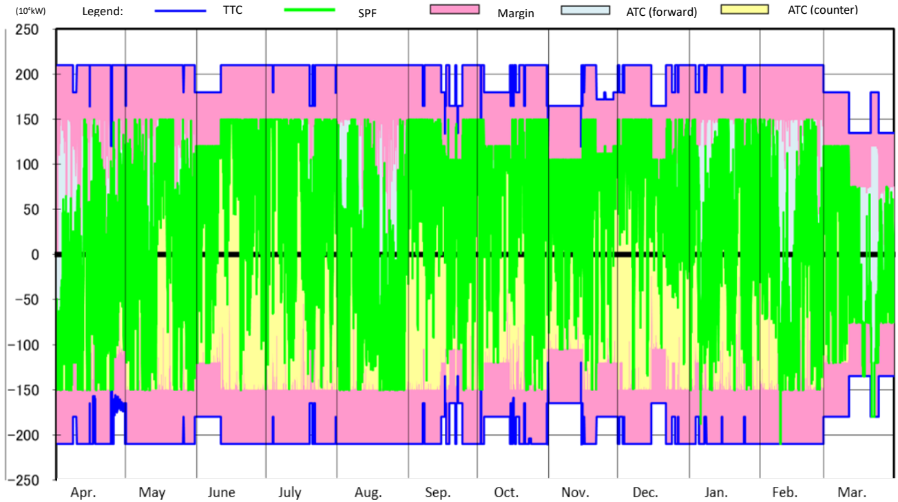
Figure 2-12: Actual ATC for interconnection facilities between Tokyo and Chubu (Sakuma, Shin Shinano and Higashi Shimizu and Hida–Shinano F.C.)
