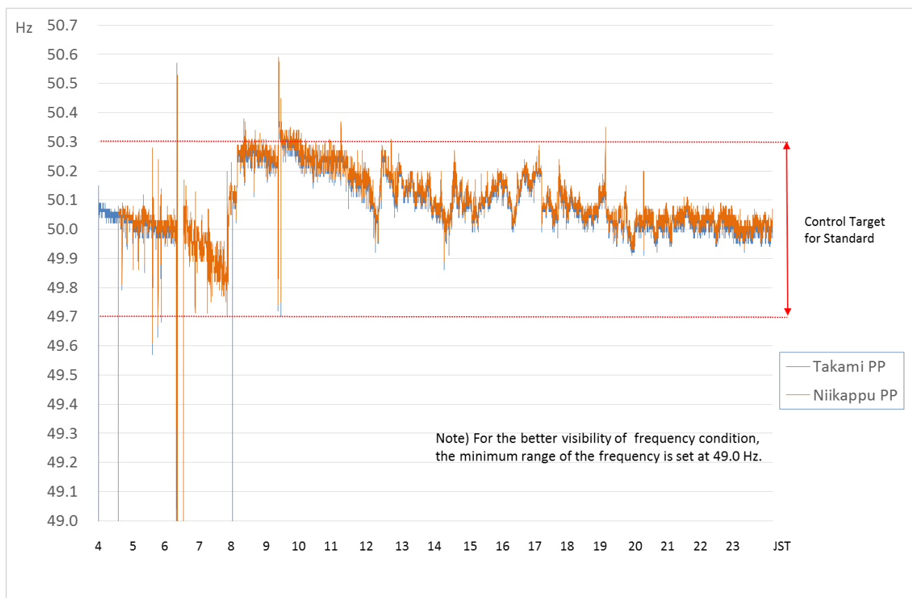
Figure 8 Bus Frequency at Takami Power Plant and Niikappu Power Plant of Hokkaido EPCO on Sep. 6, 2018 (Hz; sampling in every 3 seconds from 4:00 to 24:00 JST. Prepared anew from materials of Investigation Committee on the Major Blackout by the 2018 Hokkaido Eastern Iburi Earthquake by OCCTO)
