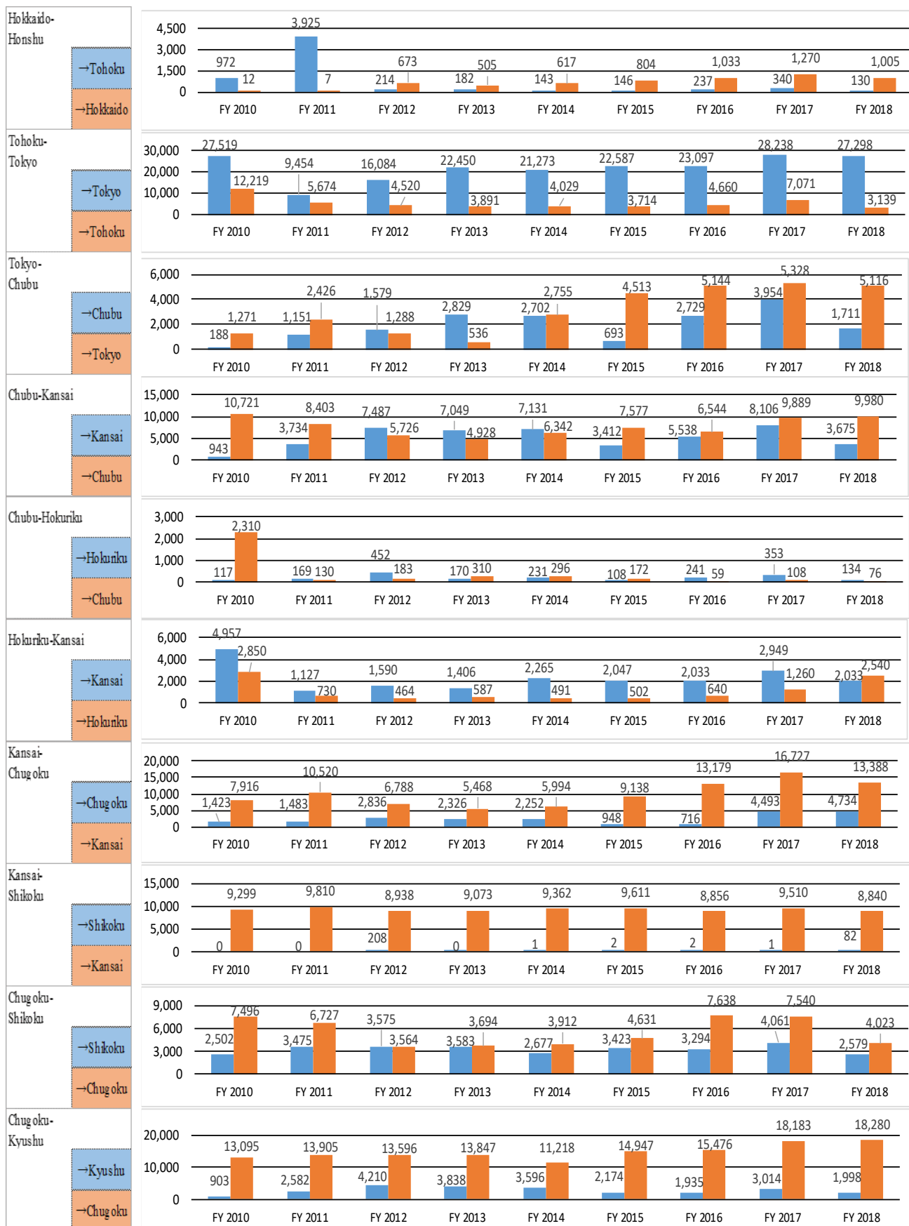
Figure 2-4: Annual Utilization of Cross-regional Interconnection Lines for Regional Service Areas (FY 2010–2018)
