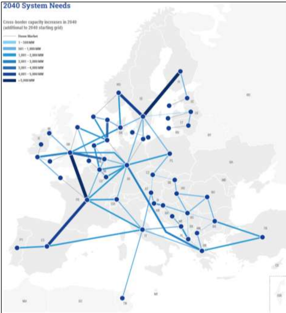
Figure 3.1 – Opportunities for increases in cross-border capacity and hybrid offshore corridors in 2040, additional to the 2030 grid for cross-border transmission.
